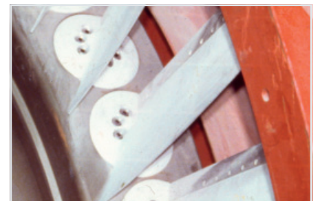
Old fan without cover plates
