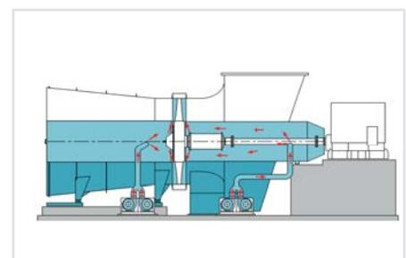
Seal air principles applied to a single stage axial fan
