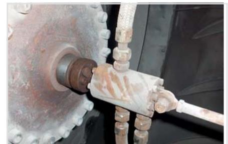
Example of corrosion of rotating oil seal and hub cover.
