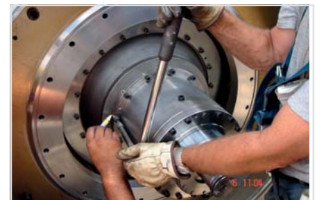
Mounting of the hydraulic cylinder.
