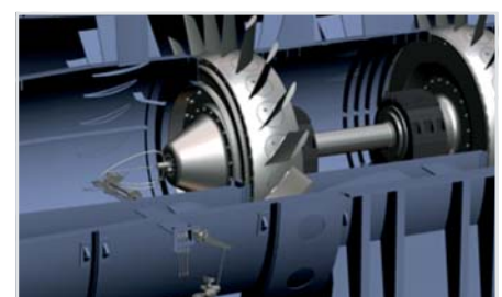
The actuator is placed on the outside of the fan moving the external regulating arm and changing the position of the hydraulic cylinder.
