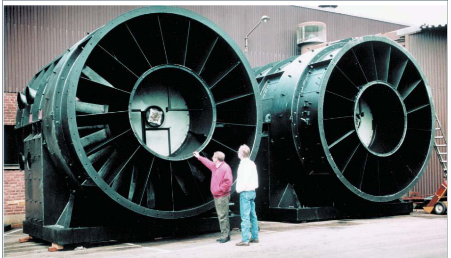
4m dia axial fans supplied to the Channel Tunnel. Motor Power 900kW. Air Flow 300 m 3 /sec. Blade pitch control during operation. 100% reversibility.
