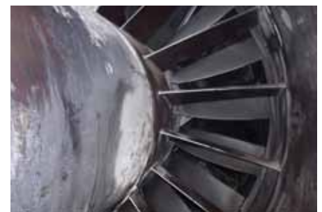
New super high pressure blade profiles and guide vanes
