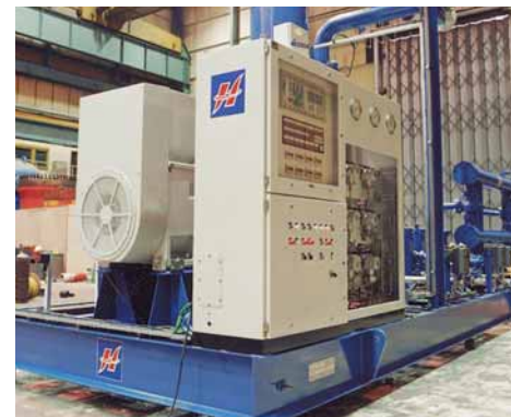
VCM recycle gas compressor with hazardous area control panel for petrochemical industry.
