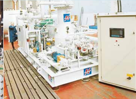
Fuel gas compressor for Boots pharmaceutical site, UK.
