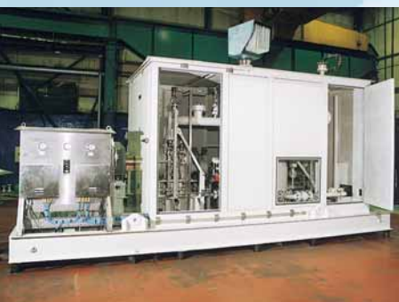
Oil injected set complete with acoustic treatment.
