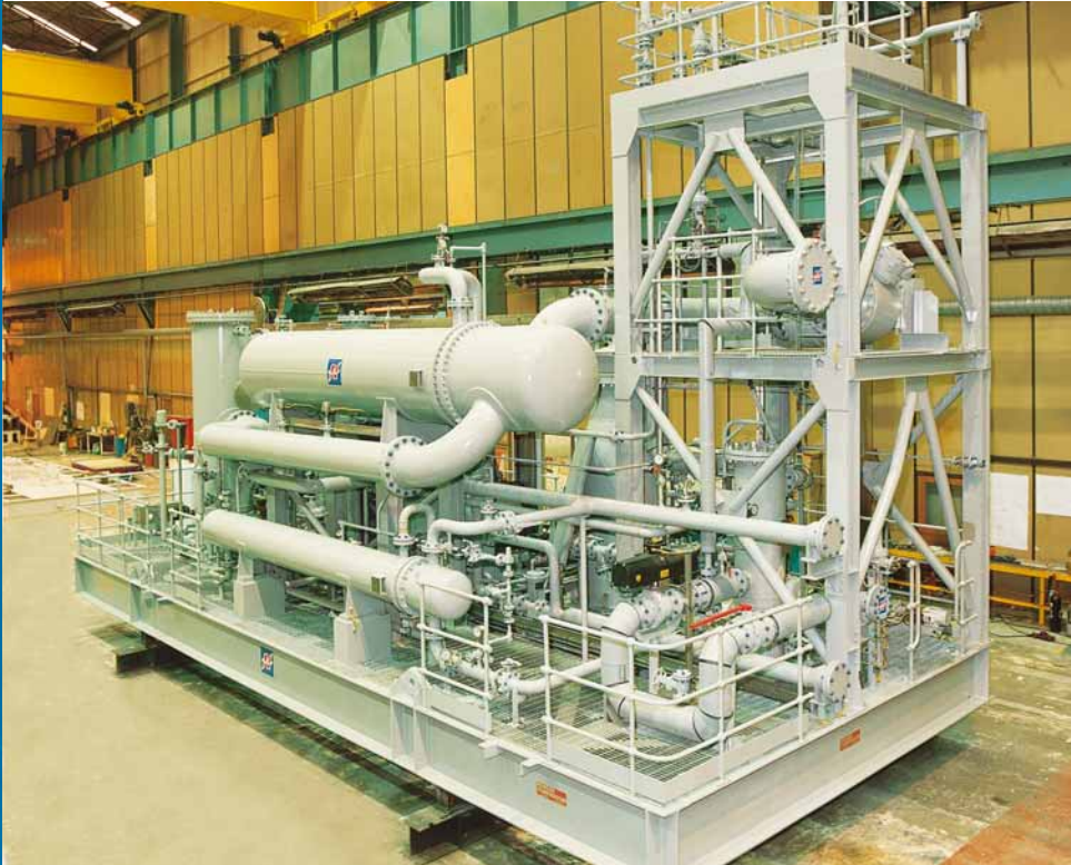
LP gas booster compressor on hydrocarbon service on BP Amoco Schiehallion FPSO
