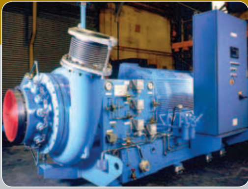
High Efficiency Howden Donkin Turbo Compressor Centrifugal Turbo Impeller
