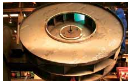
Impeller for revamping a cement plant pre-heater ID fan
