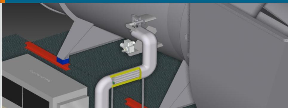
New thermal insulation ensures adequate oil flow at cold ambient temperatures.
